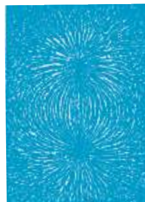
FIGURE 5.2 The arrangement of iron filings surrounding a bar magnet. The pattern mimics magnetic field lines. The pattern suggests that the bar magnet is a magnetic dipole.
