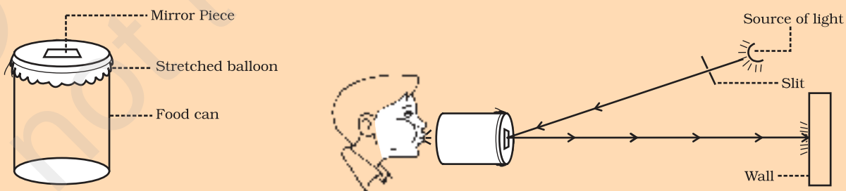
Fig. 12.4: A beam of light from a light source is made to fall on a mirror. The reflected light is falling on the wall.
